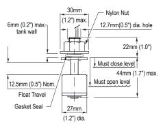
Thread sizes RSF53/4/6 M12x1.75 Thread Also available with 1/8" NPT Thread
